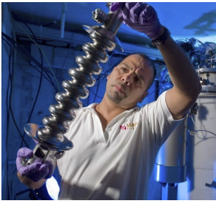
Figure 1: a) Bare 3.9 GHz cavity, b) Module solid model showing the very small cavities relative to the module.
