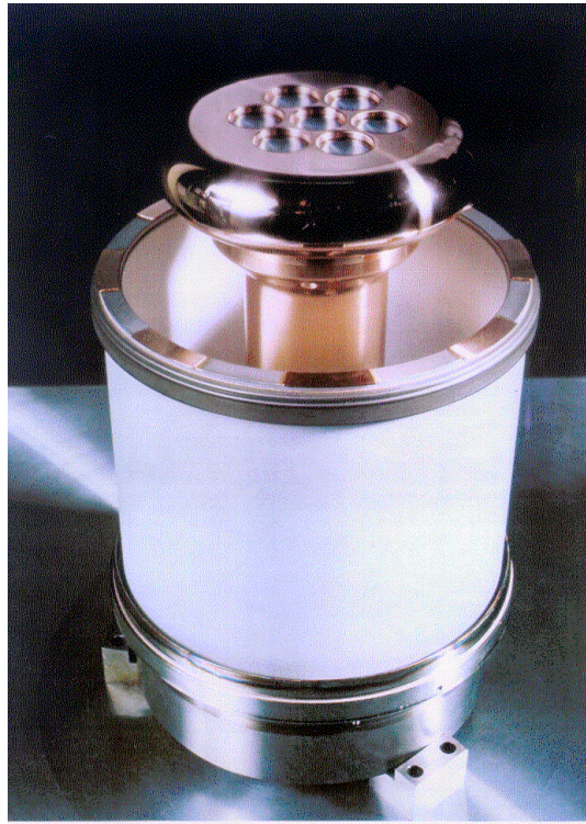
Figure 3.3.1: Cathode of the multibeam klystron.
