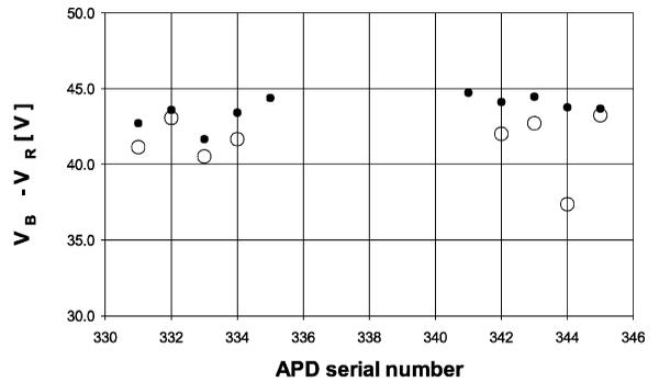
Fig. 7. Distance of bias voltage for a gain of 50 to breakdown voltage for an APD before (dots) and after irradiation (circles).
