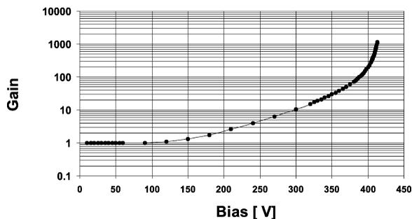
Fig. 2. Gain vs. bias voltage. The gain is 50 at about 370 V.
