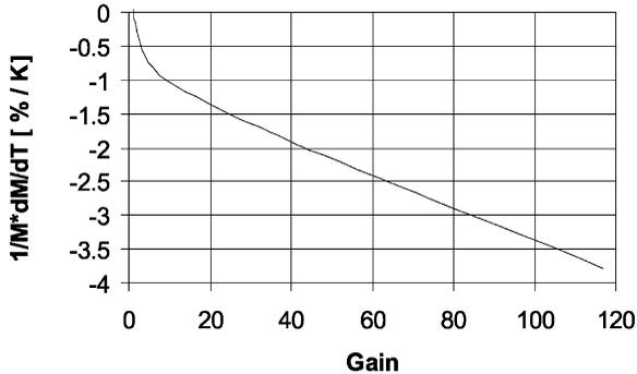
Fig. 4. Change of gain with the operation temperature.
