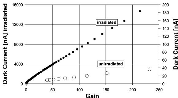
Fig. 8. Dark current vs. gain for an APD before and after irradiation.
