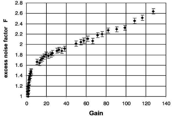
Fig. 5. Excess noise factor  $F$  vs. gain.
