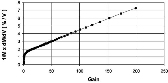
Fig. 3. Change of gain with the bias voltage.
