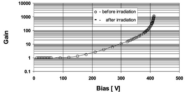
Fig. 6. Gain vs. bias voltage before and after an irradiation with protons.
