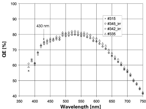
Fig. 9. Quantum efficiency vs. wavelength for two unirradiated and two irradiated APDs.
