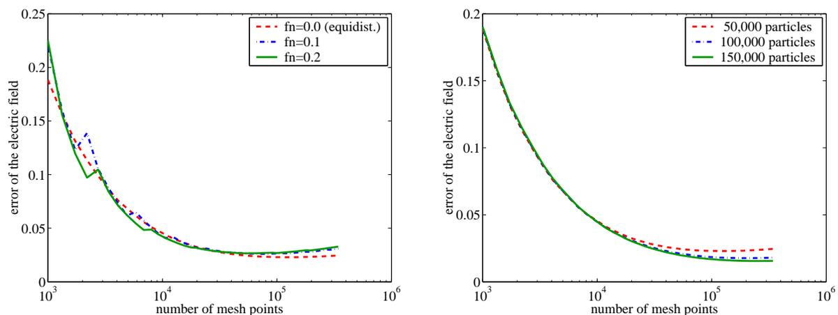
**Figure 2.** Error of the electric field for uniformly distributed particles in a sphere: Comparison of different meshes depending on parameter  $fn$  performed with 50,000 particles (left), comparison of different numbers of particles on an equidistant mesh with  $fn = 0.0$ .
