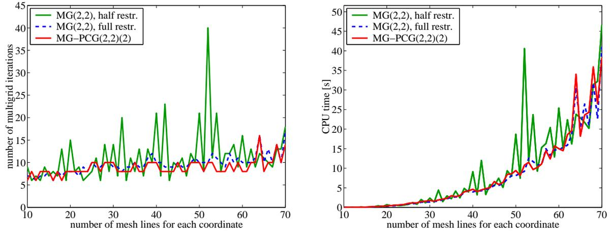
**Figure 5.** Influence of the choice of multigrid parameters to the performance of the space-charge routine: the number of multigrid iterations until the residual is less than  $10^{-6}$  in the maximum norm (left), the related CPU times measured on a 800 MHz Pentium PC (right). The calculations have been performed with a spherical bunch of 50,000 particles on a non-equidistant grid with  $fn = 0.2$ , where the particles have a Gaussian distribution.
