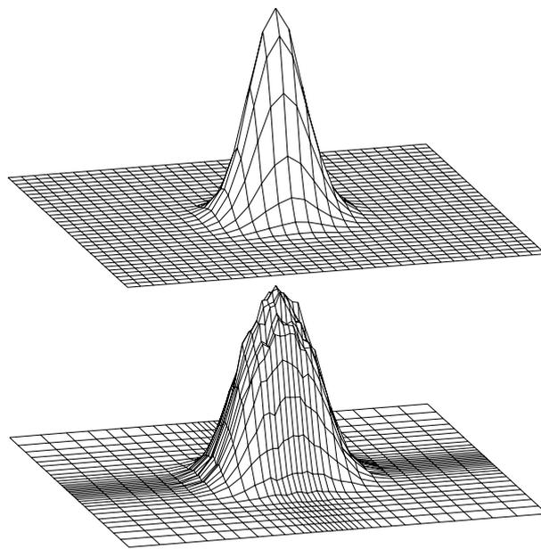
**Figure 1.** Mesh line positions ( $(x, y)$ -plane) for a Gaussian charge density with  $fn = 0$  (top) and  $fn = 0.2$  (bottom). The vertical axis shows the total charge in each mesh box, where the height of the top has been normalized in both plots.
