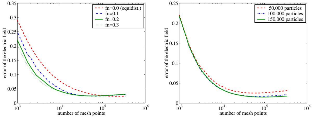
**Figure 4.** Error of the electric field for Gaussian distributed particles in a sphere: Comparison of different meshes depending on parameter  $fn$  performed with 50,000 particles (left), comparison of different number of particles on a non-equidistant mesh with  $fn = 0.2$ .
