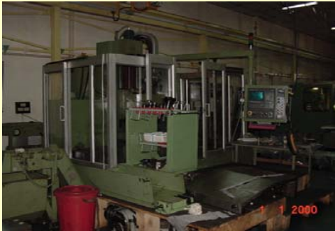
CNC BED TYPE VERTICAL MILLING VMC 800 MACHINE (M/S HMT), Table Area: 800X500 mm, Accuracy: 0.015 mm
