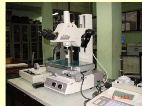
NIKON MEASUROSCOPE MAGNIFICATION 1000 X
