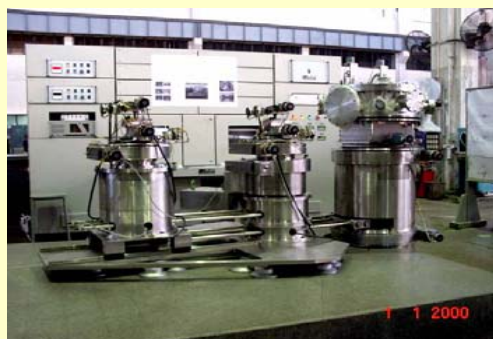
Experimental Station For EXAFS Synchrotron Beam Line (Indus-II)
