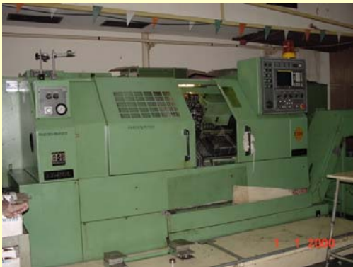
CNC LATHE WITH INCLINED & HYDRAULICALLY OPERATED CHUCK, LT-20
