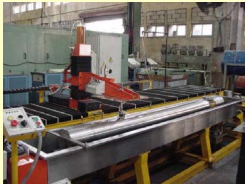
SCANNER FOR UT (M/S INTEGRATED) Size: 5215X1505X1483 mm.
