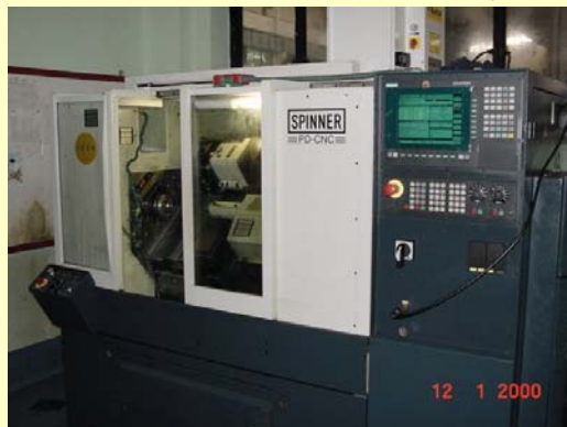
CNC, Ultra Precision, Slant Bed Lathe, Length : 400 mm Accuracy : 0.002 mm
