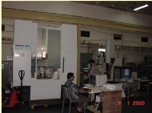
CNC 5 AXES BORING & MILLING MACHINE Table Area: 600X600 mm, Positional Accuracy: 0.01 mm
