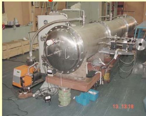
6.65m Off Plane Eagle Mount Spectrometer, CAT-INDUS-I, Wavelength Resolution 0.01 \text{ \AA} .
