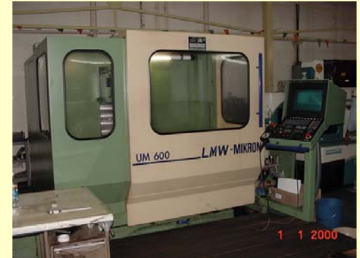
CNC Universal Boring And Milling Machine Table Area : 900X530 mm, Accuracy: 0.010 mm
