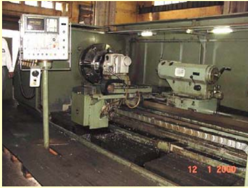
CNC Heavy Duty Spindle, BECO Lathe Turning Length: 3200 mm, Accuracy: 0.010mm
