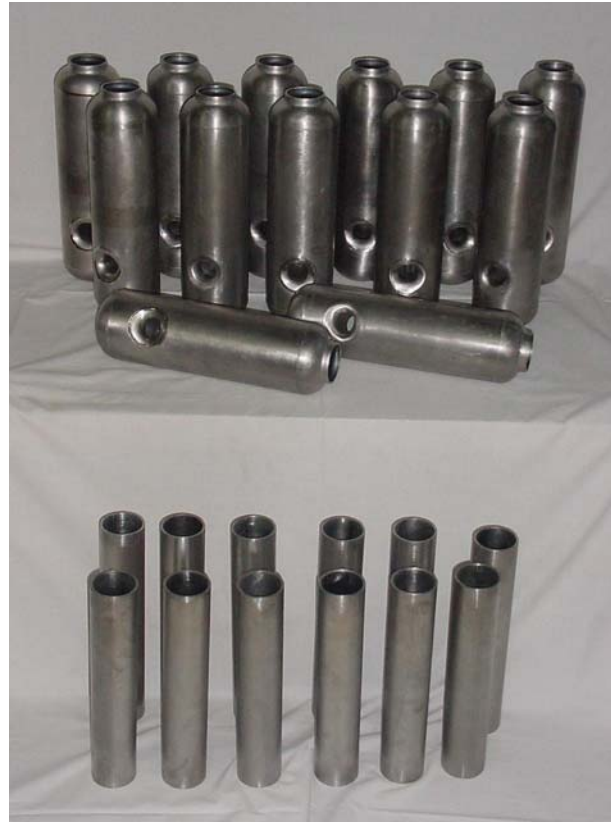
Drift Tubes (top) and Loading Arms (bottom)
