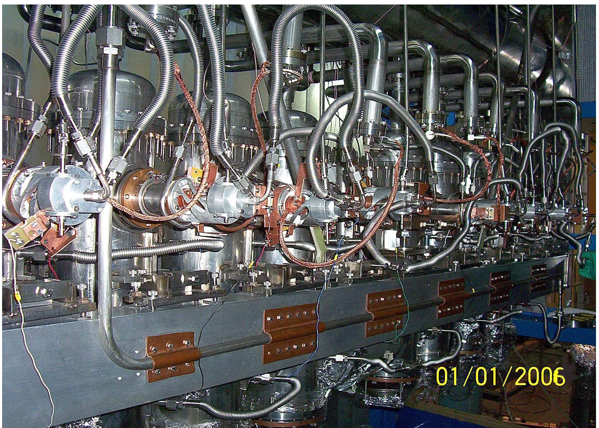
8 QWRs and superconducting solenoid in Linac module 1
