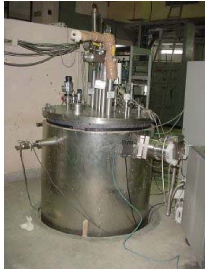
Vertical Test Cryostat
