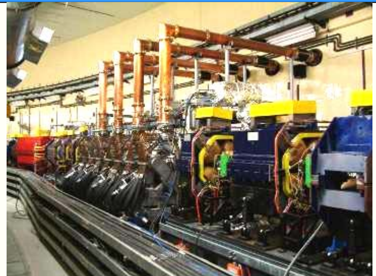
RF Cavities installed in Indus-2 Ring
